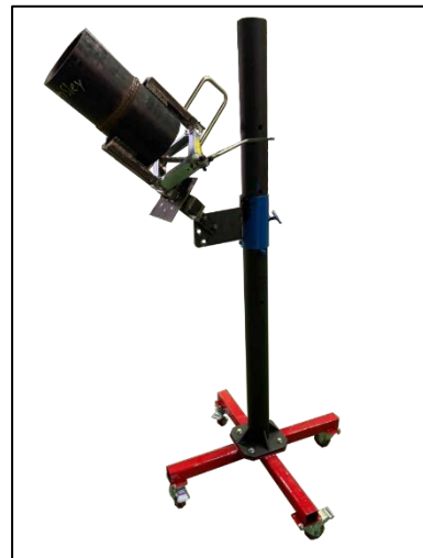
Rajah 3: Smart Welding Jig (SWJ)
